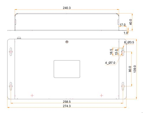
Tolerance: ±0.3 Unit: mm
