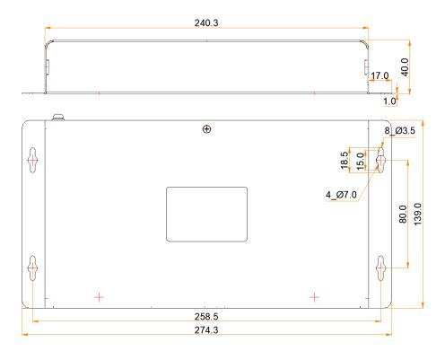
Tolerance: ±0.3 Unit: mm
