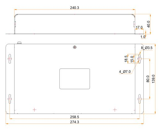
Tolerance: ±0.3 Unit: mm
