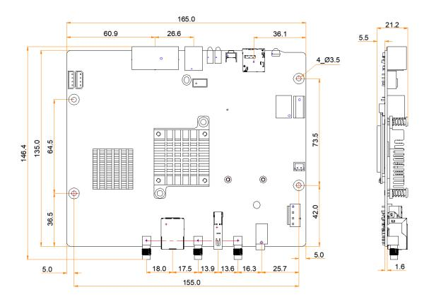
Tolerance: ±0.3 Unit: mm
