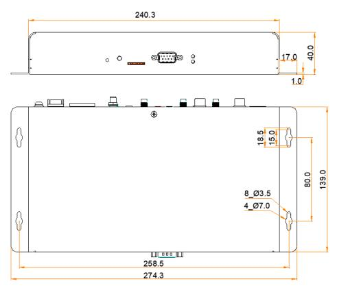
Tolerance: ±0.3 Unit: mm
