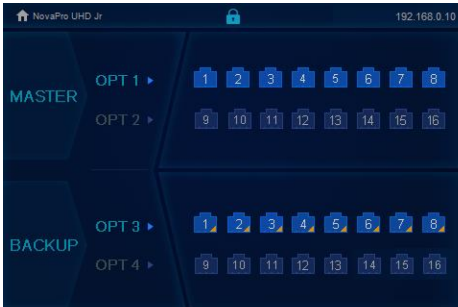
Figure 4-3 Optical fiber port statuses – Hot backup
