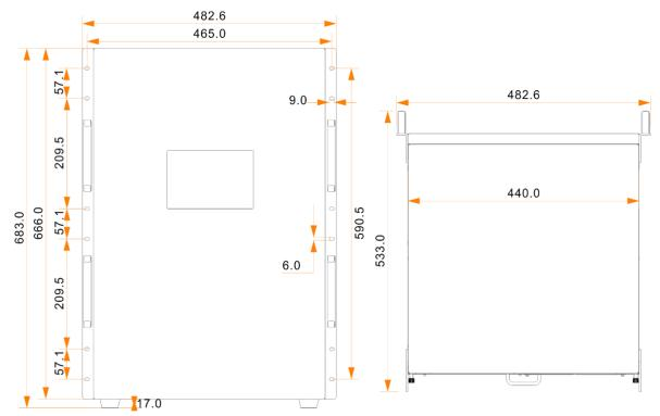
Tolerance: ±0.5 Unit: mm
