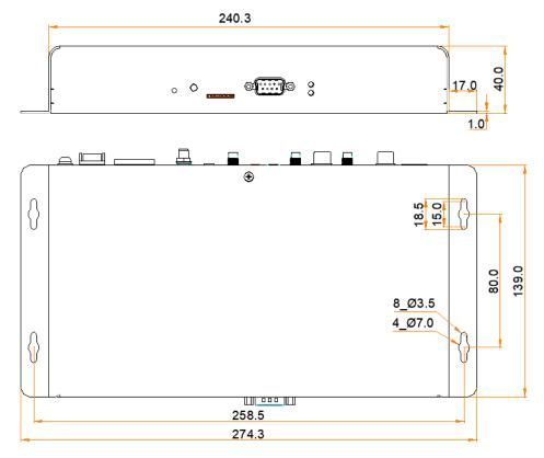
Tolerance: ±0.3 Unit: mm
