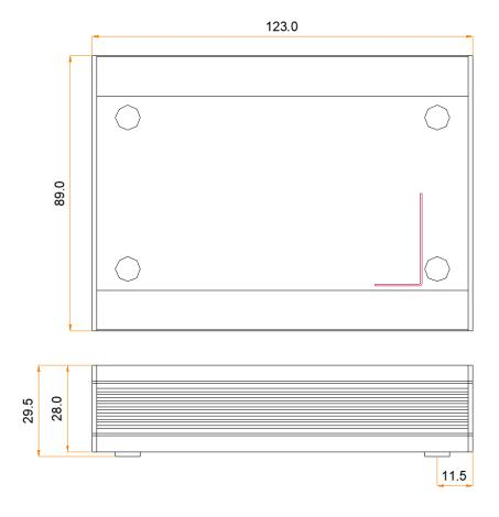
Tolerance: ±0.3 Unit: mm
