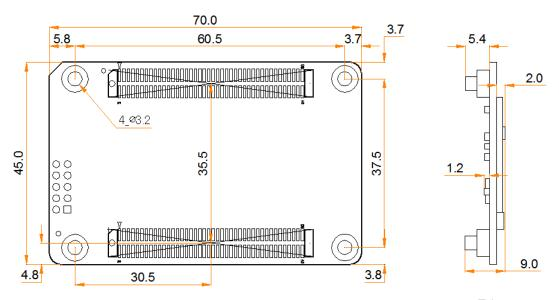
Tolerance: ±0.3 Unit: mm
