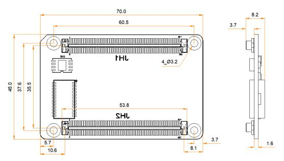
Tolerance: ±0.3 Unit: mm
