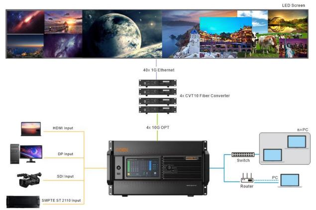
This diagram is an example of four input cards and one MX\_4x10G\_Fiber output card installed on an MX6000 Pro. The actual application may vary.
