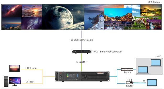
This diagram is an example of two input cards and one CX\_1x40G\_Fiber output card installed on an MX2000 Pro. The actual application may vary.
