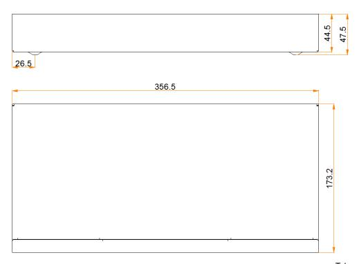
Tolerance: ±0.3 Unit: mm
