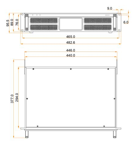
Tolerance: ±0.3 Unit: mm
