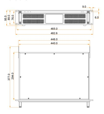
Tolerance: ±0.3 Unit: mm
