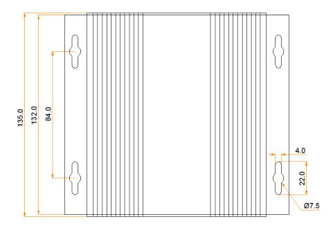
Tolerance: ±0.3 Unit: mm
