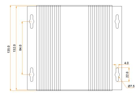
Tolerance: ±0.3 Unit: mm
