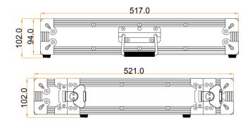
Tolerance: ±5 Unit: mm
