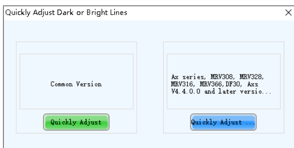
Figure 6-21 Adjusting dark or bright lines
