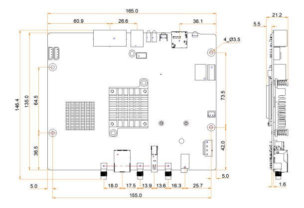
Tolerance: ±0.3 Unit: mm
