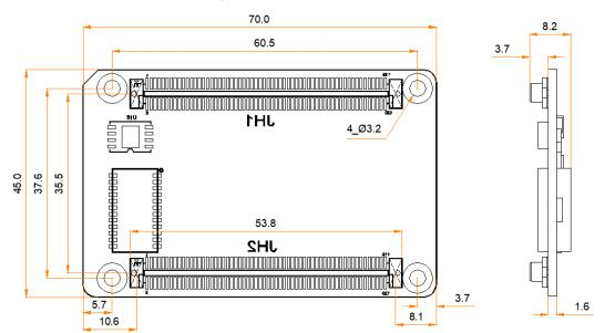
Tolerance: ±0.3 Unit: mm
