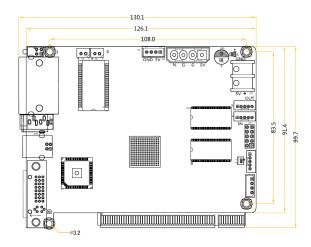
Tolerance: ±0.3 Unit: mm
