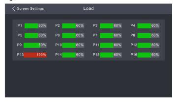
Step 2 Check the current load status of each Ethernet port of the device.
