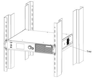
• Elevated Operating Ambient - If installed in a closed or multi-unit rack assembly, the operating ambient temperature of the rack environment may be greater than room ambient. Therefore, consideration should be given to installing the equipment in an environment compatible with the maximum ambient temperature (Tma) specified by the manufacturer.
