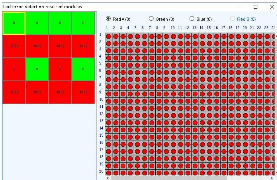
Figure 9-6 Result of the Led error detection for all the modules
