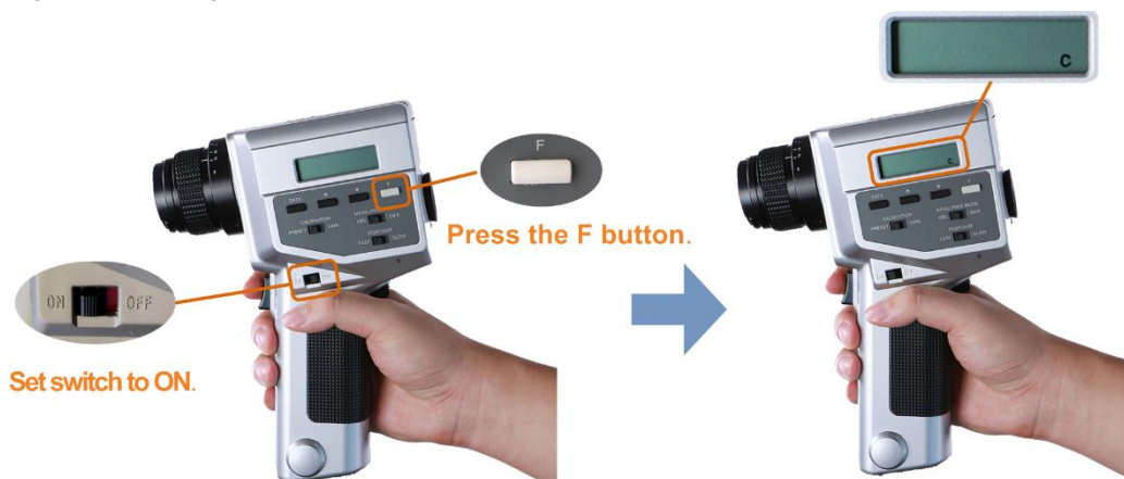
Figure 12-7 Setting CS-100A colorimeter
