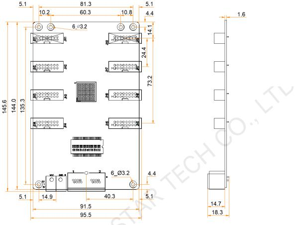
Tolerance: ±0.3 Unit: mm
