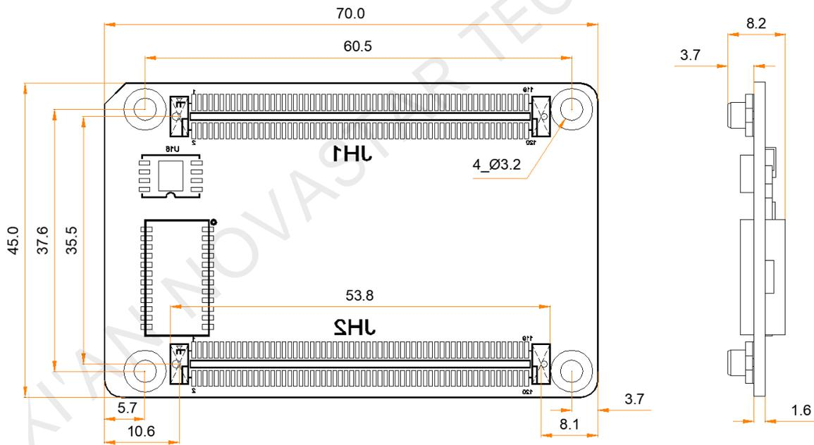
Tolerance:  $\pm 0.3$  Unit: mm
