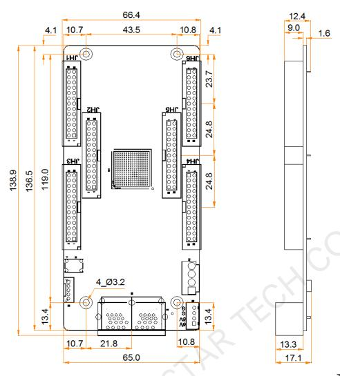
Tolerance: ±0.3 Unit: mm
