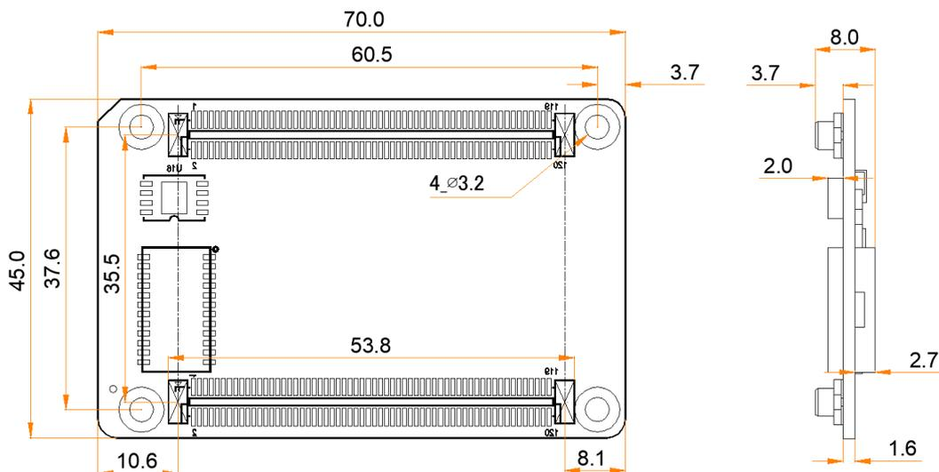
Tolerance: ±0.3 Unit: mm
