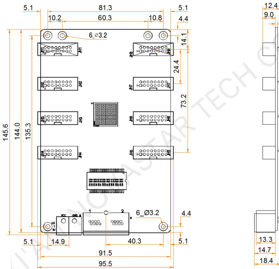
Tolerance: ±0.3 Unit: mm
