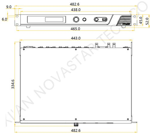
Tolerance: ±0.3 Unit: mm
