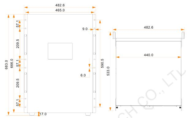
Tolerance: ±0.5 Unit: mm
