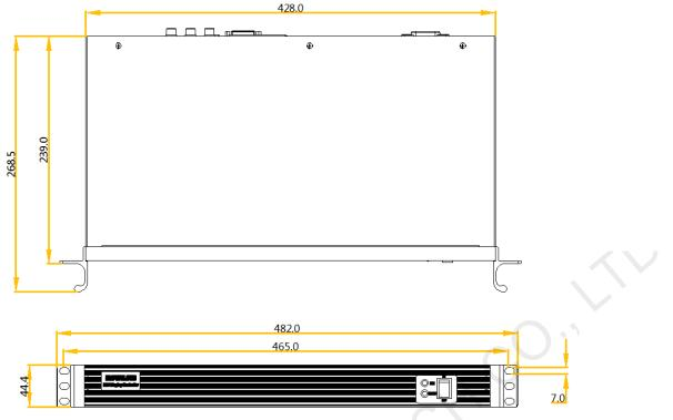
Tolerance: ±0.3 Unit: mm
