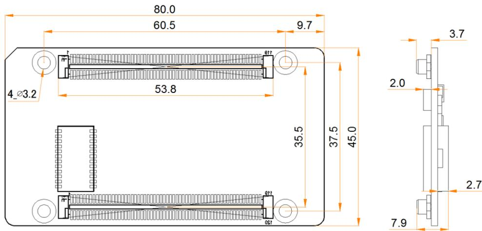
Tolerance:  $\pm 0.3$  Unit: mm
