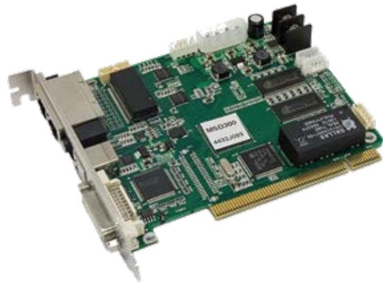
The MSD300, one of the M3 series independent controllers of NovaStar, supports video and audio input. After decoding and data processing, videos and audios can be sent to the screen via Ethernet port. A single controller supports resolutions up to 1920 X 1200@60Hz. It communicates with the computer via USB port, which is convenient to use.
