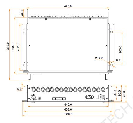
Tolerance: ±0.3 Unit: mm
