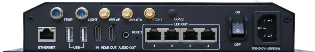
Figure 3-2 Rear panel of the TB8
