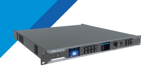
HDR Master 4K is an HDR video source generator that can transform SDR into an HDR10 video source, providing greater brightness range, richer colors and more details by using Novastar's Al dynamic range extension technology.
