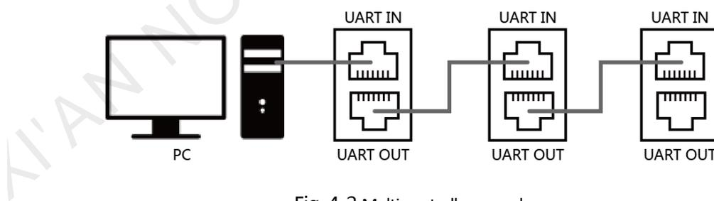
Fig. 4-2 Multi-controller cascade
